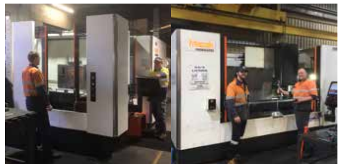
Two of the new Mazaks at GMG: the HCN-5000 twin-pallet horizontal machining centre (left) and the VTC-530/20 vertical travelling column machining centre (right).
